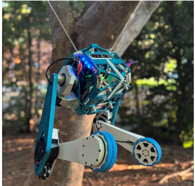
Fig. 1. Overview of WiXus, a robot that fuses a wheeled-legged system with a wire-driven system that anchors to the environment.
